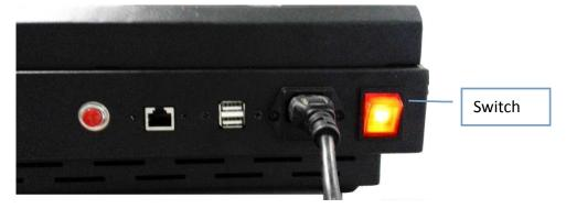
If the main switch indicator is not properly lit, check if the power cable is inserted properly.
