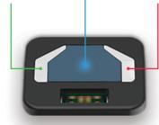
When changing modes by pressing the middle button, the selected mode will be confirmed by flashing of the correlated colour then go off again.
