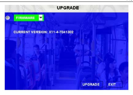
Please do not disconnect the power supply for MDVR or remove the thumb drive during firmware upgrade.
