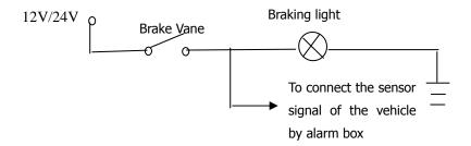
Alarm outputs are power level output. For powerful equipments, external replay is necessary. The following diagram is for how to wire the photoelectric alarm from alarm outputting.
