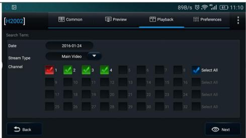
3) Enter the playback timeline interface, select the desired playback point, click **play.** Meanwhile, user can have video clips, unlock, backup and other operations.
